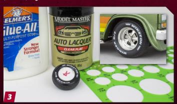
Cut discs from thick cardstock the same size as the wheel with a circle template. Attach the discs to the wheels with a small amount of white glue and then apply a wet coat of flat clear to the sidewall to protect the decals and provide an accurately dull sheen.
