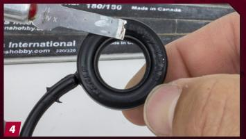
What about tires with raised-letter details molded in? Starting with a sharp No. 17 chisel blade, carefully shave off most of the raised detail. Follow with 180, 240, and 320-grit sanding sticks to smooth the sidewalls. Now, apply your decals.
