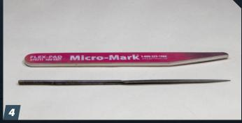
Just like plastic parts, PE requires cleanup with sanding sticks or files. Use fine sanding sticks or files because coarse grits tend to catch and bend the metal. Typically, there is minimal material to remove and it won't take many swipes to eliminate the nubs.
