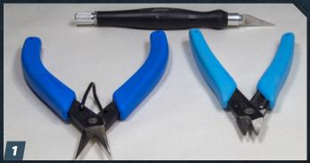
Let's start with removing the parts. The brass sheets, or frets, are typically extremely thin and the parts can be cut off with a hobby knife or specialized tools, including Xuron High Precision Scissor (No. 440) and Xuron Professional Photo Etch Scissor (No. 9180ET).
