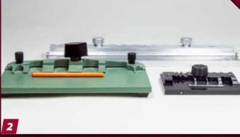
A bending tool is essential for bending parts without scoring lines or for parts that require one long, seamless bend. I use benders from UMM Models (back), JMC Hobby (right), and Mission Models (left). Each has its uses, depending on the size of the piece being shaped.
