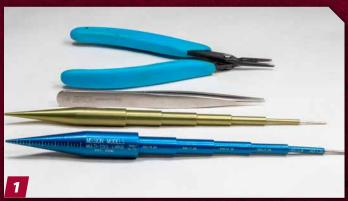
Tools can make bending PE parts easier, and, in some cases, may be necessary to nail the right shape. I commonly use (from top) Xuron Tweezer Nose Pliers (No. 450), tweezers with flat tips, and step mandrels in a couple of different sizes to form curves.
