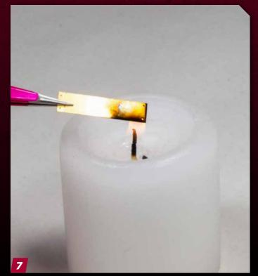
Making curves or straight bends where no score line is etched into the part can be made easier by annealing the PE part. Annealing involves heating the metal and letting it cool so it becomes more malleable. For small pieces of thin PE, a few seconds in a flame is generally all that is needed.
