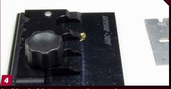
Careful study of the instructions and parts may be necessary to determine the order of bends for complex parts. In this case, a couple of bends are needed to get the main shape of a PE periscope cover, and most were easily done with the bender.
