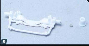
Here, the driver's side axle stub on the front crossmember was sanded down to compensate for the 0.010-inch thickness of the square of bottle cap and the 1mm thickness of the rare earth magnet. Superglue the metal square to the stub and round the corners with 320-grit sandpaper until the wheel cap fits smoothly.
