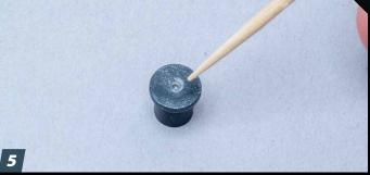
Superglue the magnets inside the wheel caps. To accomplish this, drill a small hole in the end of the cap. Add a drop of superglue from the outside after the magnet is inserted into the cap and resting flat inside. Now, finish your wheel as per the instructions. **FSM**
