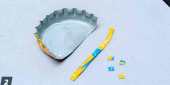
First, take your metal bottle cap and cut a strip from it as wide as the diameter of the axle. Then, cut it into squares — four of them to be exact.
