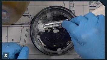
Use tweezers to fully submerge the chrome-plated parts in the Liquid Plumr. They will probably float to some extent, but the important part is to make sure the Liquid Plumr coats the parts.
