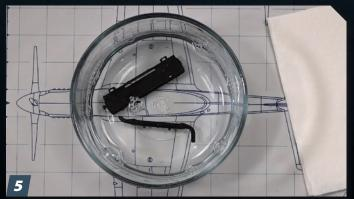
Ta-da! The chrome has disappeared from the parts. Fill the other bowl with water and thoroughly rinse the parts. You may need to scrape with a toothpick or scrub with a toothbrush to eliminate stubborn chrome in nooks and crannies.
