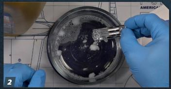
Pour the Liquid Plumr into one of the glass bowls. Do this slowly to avoid splashes or spills. Carefully place the chrome-plated parts in the bowl. If you don't have a big enough vessel to hold all the parts, you may have to strip the chrome in batches.
