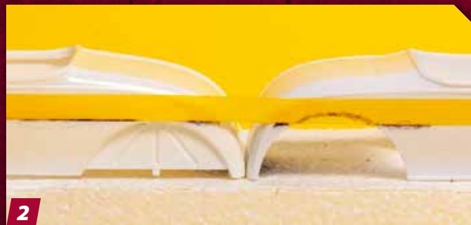
2 Mark the correct height for the top of the fender opening with 1/8-inch-wide tape from the AMT body onto the Revell body. If you don't have the AMT body, you can approximate this step using the body on the right in the photo as a reference.
