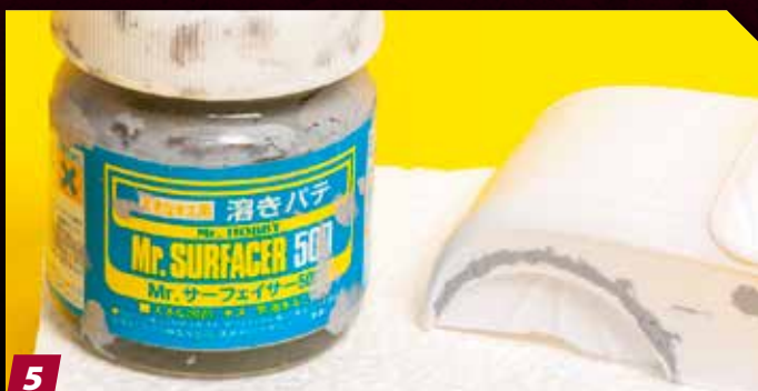
5 Smooth the body along the fender openings on each side to achieve a flush surface. Use Mr. Surfacer 500 to fill joints where the two parts meet. After sanding, prime the body, check for any flaws, and repeat the filler/sand/prime process until you are satisfied with the result.
