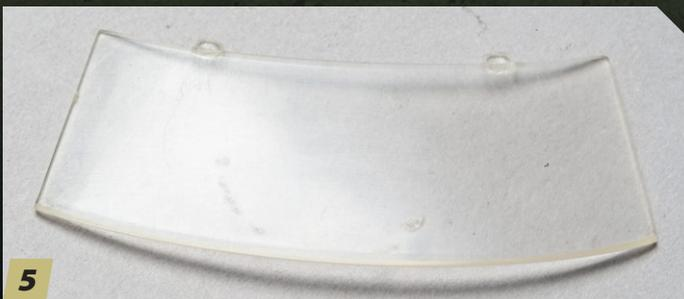
**5** Progress through the rest of your sandpaper, up to 2000 grit, and the damage should be gone. The plastic is uniformly hazy but not yet clear. If there are moderate or large scratches visible, go back to a coarser grit and eliminate them with another round of sanding. You could go directly to polishing compounds at this point, but I recommend continuing with polishing cloths first.
