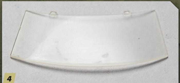
**4** Move on to 600-grit sandpaper, sanding the area you've previously worked. Notice the sanded area has been expanded somewhat. Since the grits used are so mild, don't be afraid of over-sanding, especially as the grits become finer. Use each grit until it removes all the scratches from the previous one.
