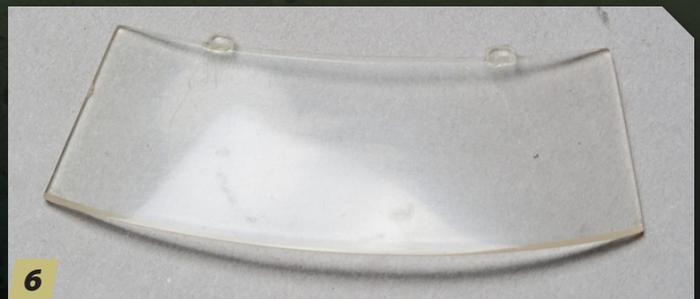
**6** After working through the polishing cloths up to 12000 grit, it's time to apply a polishing compound, as directed, with a soft cloth. The imperfections that can be seen now are on the other side. In addition to the tire damage, there are some scratches up by the mounting tabs on the top edge. Now, it's time to flip it over and perform the same process to fix the marks on the other side.
