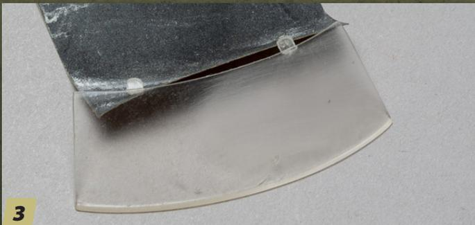
**3** Start with the deepest and sand the defect smooth with 400-grit sandpaper. Only sand the area around the repair, not the whole part. It might be tempting to use a coarser grit to get to the bottom of the depression quicker, but anything more than 400 will create scratches that will take longer to remove in subsequent steps.
