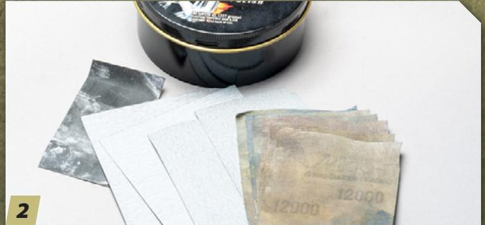
**2** You'll need wet or dry sandpaper in 400, 600, 1000, 1500, and 2000 grits; a set of polishing cloths or pads from 3200, 3600, 4000, 6000, 8000, and 12000 sheets; and polishing compound and a soft cloth to apply it. For the polishing compound, any brand will work; Meguiar's, Tamiya, and Novus are excellent polishes that I regularly use.
