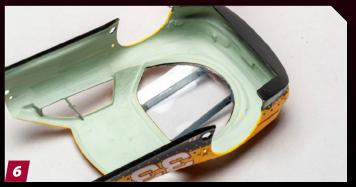
A bead of R/C 560 Canopy Glue was applied to the inside perimeter from the bottle, and I cleaned up the excess with a damp cotton swab and paper towel. The wax applied earlier helped make cleaning up the Canopy Glue a breeze.
