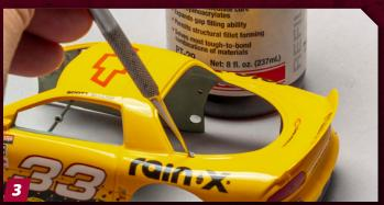
Apply a small amount of accelerator to a few spots around the window opening, not directly to the clear part — it can craze the plastic or affect the paint. Let the accelerator dry for several minutes; the longer you wait, the more time you have to position the part. The less time you wait, the quicker the superglue will cure.
