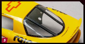
After gluing the other side near the B-pillar, I removed the tape and placed a drop of superglue to the rear of the window with the pin. I could have called it done at this point, but I wanted a bit more reinforcement.
