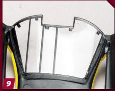
Letting the accelerator dry longer allowed the superglue to flow in deeper before it "kicked off" but also prevented it from seeping through to the car exterior. The superglue cured within less than a minute, but I let it sit for a good five minutes before I buffed my fingerprints off the glass.
