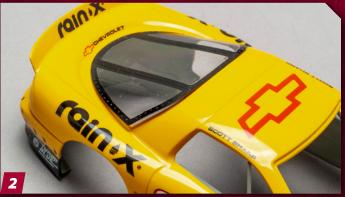
You can see here the Camaro window is wider than the opening. Superglue is one of the best ways to get it to fit. The window has been sanded and reshaped to fit as well as possible, but it is simply too wide where it meets the B-pillars.
