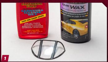
Wax both sides of the clear part, let it dry, and buff it out. This acts as a protectant in case the superglue creates any fog. You can buff it out easier off of wax than raw plastic. If you painted your clear part, use a liquid wax after painting and buff softly to avoid removing paint.
