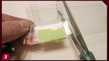
Attach the kit windshield to the cellphone screen protector with masking tape. Using a heavy pair of scissors, cut the cellphone protector along the edge of the windshield, fracturing the glass naturally. Important: Leave the film screen protector in place.
