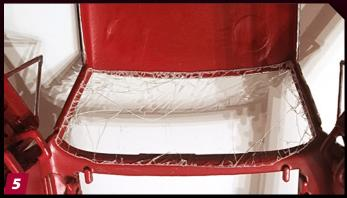
After test-fitting and final trimming, the windshield is ready to be glued in. Superglue is the way to go. I prefer Loctite 242 or 454, but any medium or medium-thick viscosity superglue will work. Do not use a thin superglue because it runs too easily. Work slowly.
