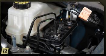
Antilock brake systems often have different configurations than what we've explored so far. For example, this is the under-hood braking system of a 2024 Ford Mustang GT. You would really blow away the troops if you reproduced this in miniature, but we need a full-detail S650 Mustang GT model kit first! **FSM**
