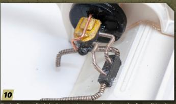
Typically, you find the booster/master cylinder on the firewall (on hot rods and pickups it's often on the underside of the floorboard). Here the equalizer/combination valve is mounted on the fender wall. Note the brake lines routed between the two components, down the fender, and (eventually) into the frame. The master cylinder cap retaining wire is modeled from fine copper wire.
