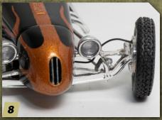
Whether drum or disc brake, make sure to leave enough extra length in your front hydraulic lines to account for the suspension moving up and down and the wheels turning right or left. Keep the routing away from suspension pieces, such as radius rods, tie rods, and drag links.
