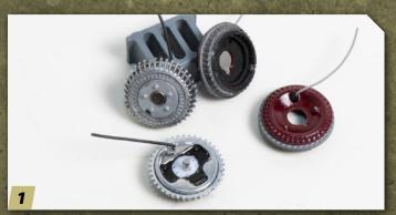
You have two predominant types of brakes — drum and disc. On the left, here's the most common hot-rod drum-brake system (1940-48 Ford hydraulic) paired with mid-20th century ribbed Buick drums. On the right is the rare (among full-size hot rods) Kinmont brake system from Replicas & Miniatures Co. of Maryland.
