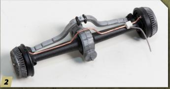
At the rear, hard tubing (modeled with copper wire) connects the drum brakes to a junction box mounted on the rear axle (white). From the junction box, a flexible hydraulic line connects to the chassis. Paint the tubing and junction box semigloss black or metallic gray after installation.
