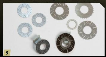
Photo-etched metal parts have become a prevalent option for brakes. On top, you see the basic parts and the complete assemblies below. On the right is a modern-era disc brake — much larger than the vintage on the left. Also, on modern cars and trucks, the front rotors are typically larger than the rears.
