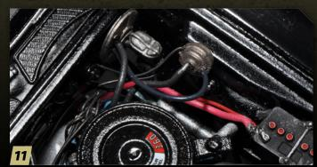
Add a scale hose between the power brake booster (top center of image) and the rear of the engine intake manifold. This line supplies vacuum to support the brake booster. In this image, a second vacuum line runs from the power brake booster to the Speed Control Servo on a 1974 Plymouth Road Runner.
