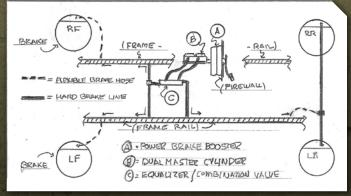
Here's a diagram of a typical brake system. Details vary by make and model of vehicle, so for a precise replica, consult a shop manual for your vehicle or find a 1/1 scale example of your subject and take pictures for your reference.
