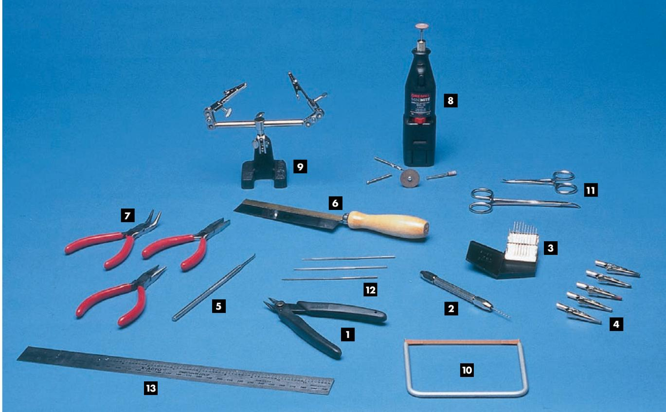
For the intermediate builder, a few handy gadgets can make all the difference. Many are merely improvements on basic tools: For example, you can use a “third hand” and a variety of clamps instead of clothespins (perhaps), or a pin vise to boldly put holes where no holes were before. The bow sander is great for working on compound-curved surfaces without flattening them. A scribe restores, repairs, or clarifies panel lines.
