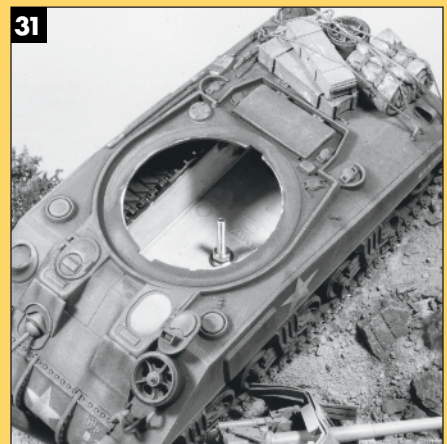
31 Scott drilled a hole in the base, pushed a bolt through, and secured the Sherman with a nut.
