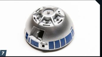
With your primer coat done, airbrush your original color. Apply thin coats, building up an even finish. Concentrate on the seams and move outward. Metallic paints tend to make imperfections stand out, so make sure your primer coat is as smooth as you can get it. **FSM**
