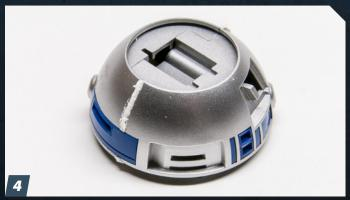
Knock down the putty with a medium-grit sanding stick and then remove the tape. There's no avoiding it: At this point, some paint is going to have to come off.
