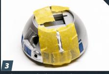
Apply putty to both seams. Place tape alongside the seam to minimize the mess. Overfill the seam because the putty will shrink when it dries. Let the putty cure completely — 24 hours will do the trick.
