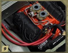
Heater hoses are sometimes a faded red color rather than black. Typically, attach heater hoses to the model's engine during its initial assembly. Attach the opposite ends of the hoses to the firewall or heater during final assembly.
