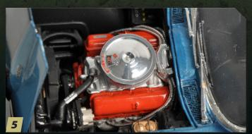
For instance, most early generation Corvette engines used special shielded ignition cables to eliminate radio static due to the noninsulating properties of the fiberglass bodies. Craft store elastic metallic thread provides a believable scale simulation.
