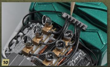
Fuel lines differ widely on each engine type. Here, six individual fuel lines run from each carburetor on this hot-rod engine to a fuel block mounted on the firewall. A single line runs between the fuel block and gas tank, routed through an electric or mechanical fuel pump.
