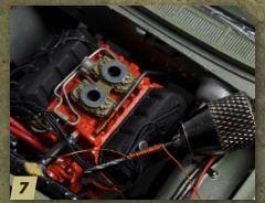
Slip the throttle return spring off the drill bit or pin and install it on the engine, running from the carb linkage to the front of the intake manifold. Use references for your specific engine to determine the correct location and color for the spring.
