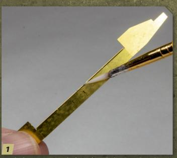
For a hedgerow cutter on the front of a tank, the seam where the pieces join needs to be strong for handling during the rest of assembly and attachment to the model. First, brush liquid flux along the seam where the solder needs to flow.
