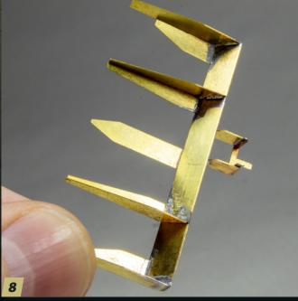
Here is the finished hedgerow cutter. While it could have been built using superglue, it likely would have come apart causing rework and unnecessary frustration. Instead, solder created nearly indestructible joins and allowed for a detailed, complex PE subassembly. **FSM**
