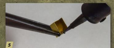
When soldering an interior join, apply flux to the seams where the sides connect. With a small amount of solder on the tip, touch the iron to the seam; the solder will flow down the join for a strong bond. This box would have likely come apart if assembled with superglue.
