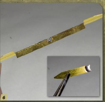
For single parts to be joined into a larger whole, you need to "tin" the parts, which means applying solder to where they will join. As before, brush flux onto both parts where the join will be and then melt a small amount of solder onto them.
