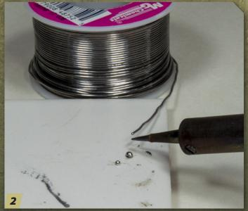
Melt small amounts of solder into several tiny beads on a hard, temperature resistant work surface. Melt these solder beads onto the tip of the iron. This method gives you greater control over the amount of solder you use rather than loading the iron tip direct from the solder spool.
