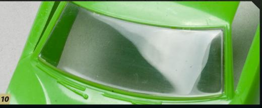
Here, I've taped the windshield in place using the mounting tabs to test-fit it inside the car body. You can use this process on any clear part, whether it's for a scale model car, airplane, helicopter, or starfighter. Just take your time and make sure to thoroughly eliminate the scratches caused by the previous sanding before moving on to the next higher grit. **FSM**
