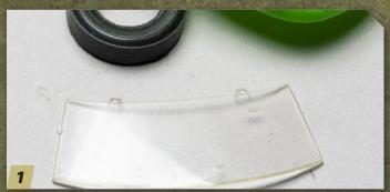
Trying to replace the windshield of a rare IMC Avenger GT-12 with plastic sheet would not yield the best fit. The thin part fits flush and has two mounting tabs molded into it. Rather than replacing it or using similar parts, you can fix it instead.
