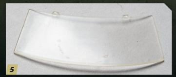
Progress through the rest of your sandpaper, up to 2000 grit, and the damage should be gone. The plastic is uniformly hazy but not yet clear. If there are moderate or large scratches visible, go back to a coarser grit and eliminate them with another round of sanding. You could go directly to polishing compounds at this point, but I recommend continuing with polishing cloths first.
