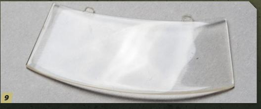
At this point, the part has been sanded thoroughly and treated with polishing compound. There is a black speck I suspect was introduced during molding that I'm willing to live with — a stone kicked up from a truck that nicked the windshield, let's say.
