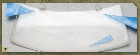
This is the inside of the windshield after wet-sanding the tire imprint with 400 grit (bottom arrow), I switched to 600-grit sandpaper to erase it entirely. Then, I switched to 1000-grit sandpaper to refine the 600-grit work and also began correcting the fine scratches near the tabs (top arrows). No need to go after those fine marks with a larger grit and cause more work or potentially more damage.
