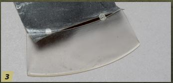
Start with the deepest and sand the defect smooth with 400-grit sandpaper. Only sand the area around the repair, not the whole part. It might be tempting to use a coarser grit to get to the bottom of the depression quicker, but anything more than 400 will create scratches that will take longer to remove in subsequent steps.
