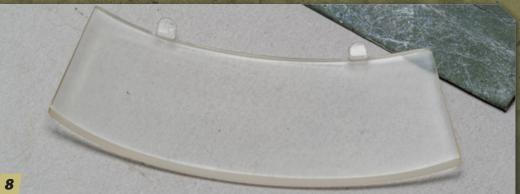
I treated the entire inside face of the windshield with 1500-grit sandpaper until it had an even sheen. I made sure there were no shiny depressions and no significant, deep scratches that stood out. Once satisfied, it was time to move on to 2000-grit sandpaper and then the finer polishing cloths.
