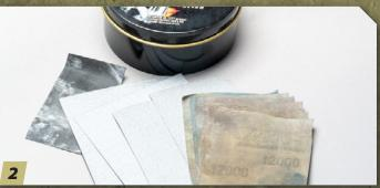
You'll need wet or dry sandpaper in 400, 600, 1000, 1500, and 2000 grits; a set of polishing cloths or pads from 3200, 3600, 4000, 6000, 8000, and 12000 sheets; and polishing compound and a soft cloth to apply it. For the polishing compound, any brand will work; Meguiar's, Tamiya, and Novus are excellent polishes that I regularly use.
