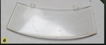
After working through the polishing cloths up to 12000 grit, it's time to apply a polishing compound, as directed, with a soft cloth. The imperfections that can be seen now are on the other side. In addition to the tire damage, there are some scratches up by the mounting tabs on the top edge. Now, it's time to flip it over and perform the same process to fix the marks on the other side.
