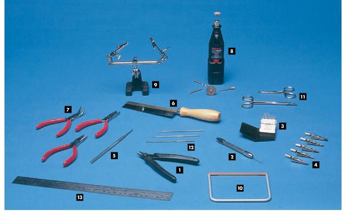
For the intermediate builder, a few handy gadgets can make all the difference. Many are merely improvements on basic tools: For example, you can use a "third hand" and a variety of clamps instead of clothespins (perhaps), or a pin vise to boldly put holes where no holes were before. The bow sander is great for working on compoundcurved surfaces without flattening them. A scriber restores, repairs, or clarifies panel lines.
